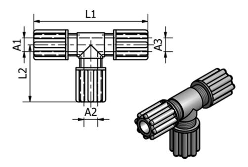
Ext. Hose Diameter A1 = 8/10Ext. Hose Diameter A2 = 8/10Ext. Hose Diameter A3 = 8/10L1 = 70L2 = 35
